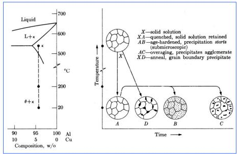
Figure illustrating the heat treating process for an Aluminum-Copper alloy
