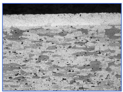
Micrograph Showing an Aluminum Alloy with a Clad layer
