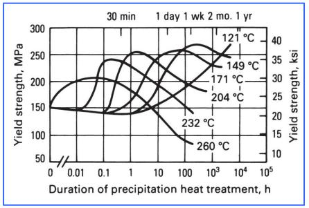
Precipitation heat treatment or artificial aging curves for solution heat treated and quenched aluminum alloy 6061 (Al-Mg-Si) show the changes that occur with increasing time at each of a series of temperatures.
