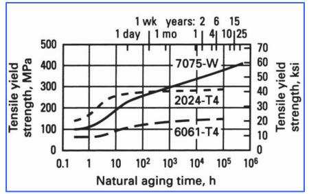
Natural aging curves for three solution heat treated aluminum alloys
